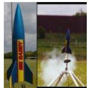
How do you get the rocket back? All model rockets are required to have some sort of "recovery system" to bring the rocket gently back to earth. Usually this will be a parachute or streamer. However, some rockets will glide back just like the space shuttle or spin down like a helicopter.
